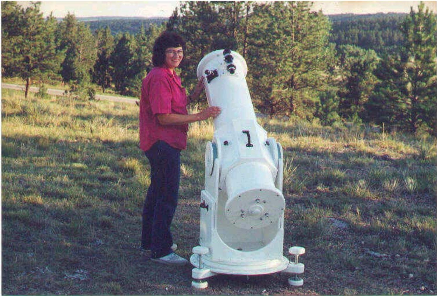
**1994-- 10" f/5.0 Dobsonian made for use at Hidden Valley Observatory. The telescope was constructed by Steve Parker and the optics fabricated by Ron Dyvig**
