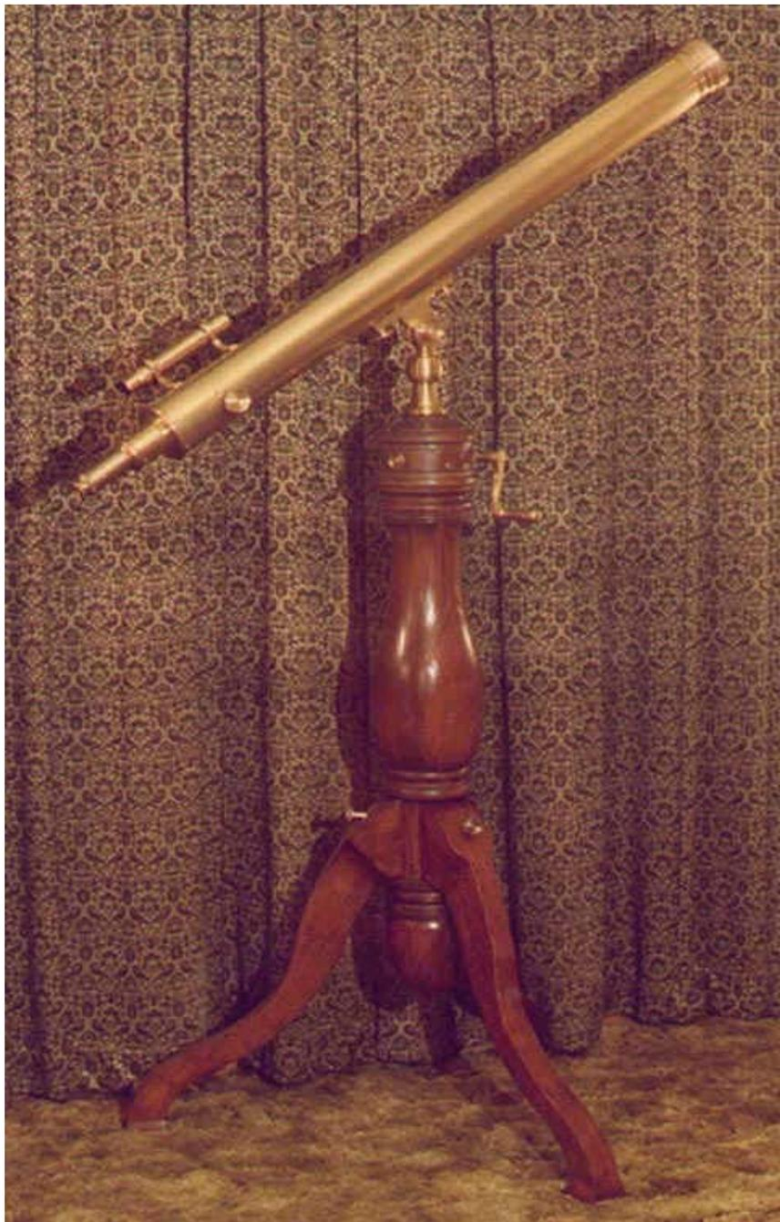
**1986--This vintage-style brass refractor used an objective lens manufactured by the A. Jaegers Co. It was featured in the December 1986 issue of Sky & Telescope magazine. This was not a replica of a particular antique instrument, rather an original design employing the methods and materials prevalent in the 19th century.**
