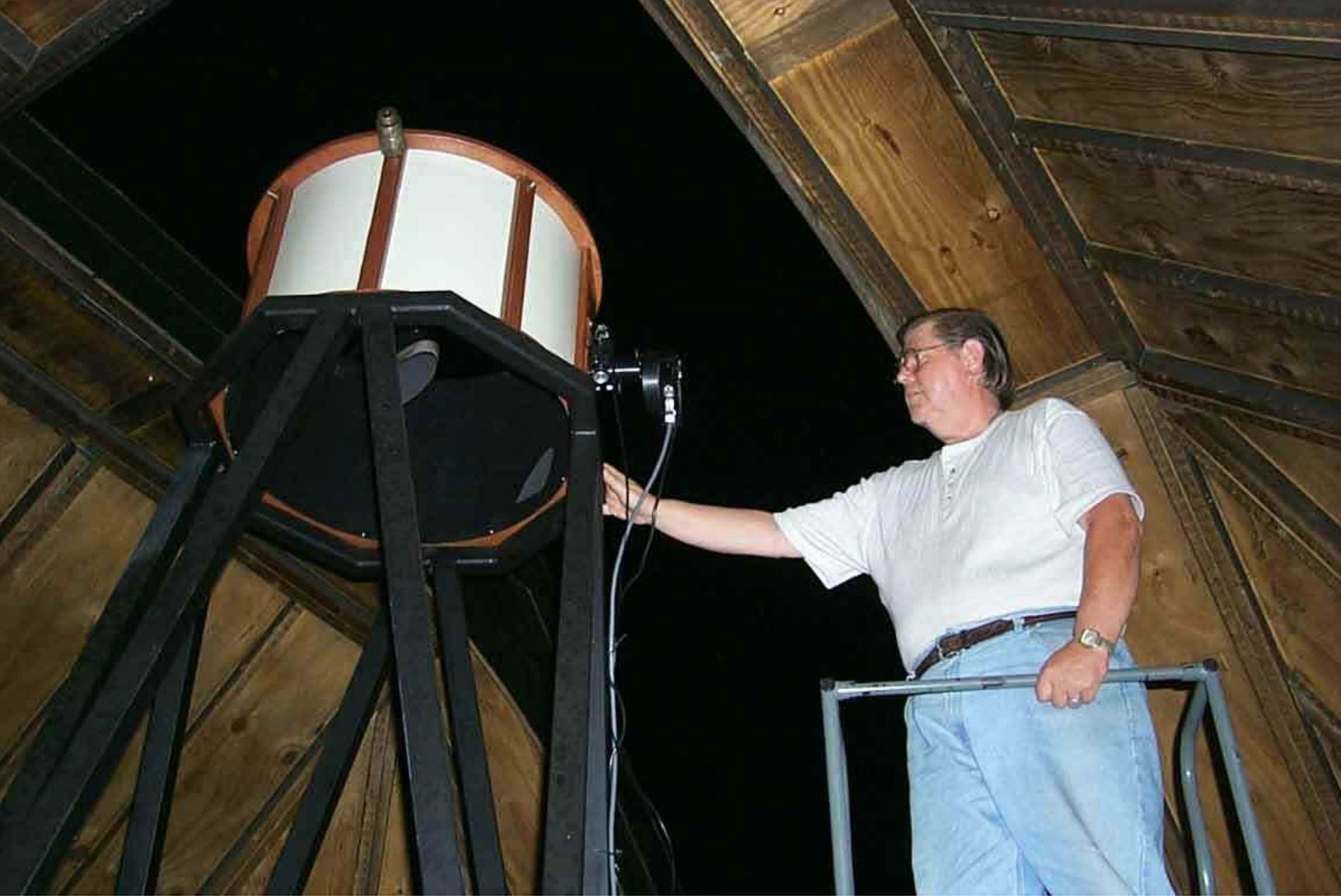
**Badlands Observatory - Image shows viewing port on upper end of the tube assembly. Ron Dyvig is on top of the stair platform adjusting the ST-8 CCD camera.**
