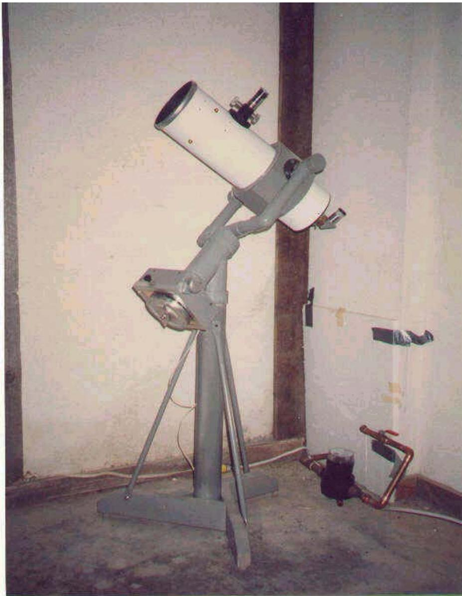
1984 -- 6" Newtonian/Cassegrain combination telescope was built for less than \$100.
