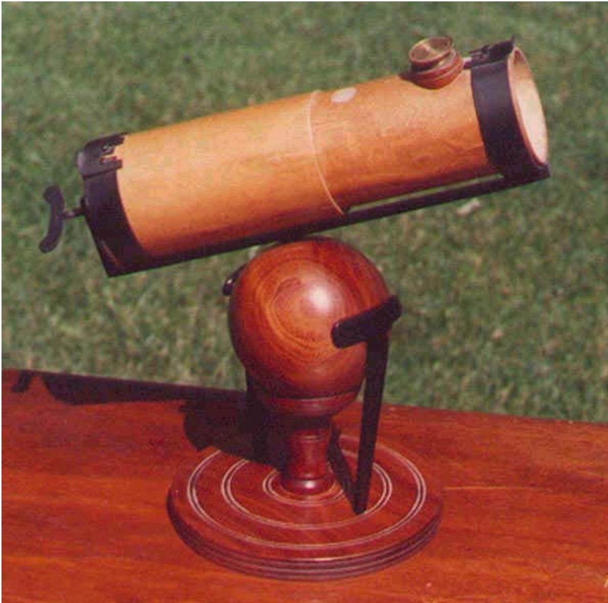
**1975--This is a replica of the first reflecting telescope invented by Sir Isaac Newton in 1668.**
